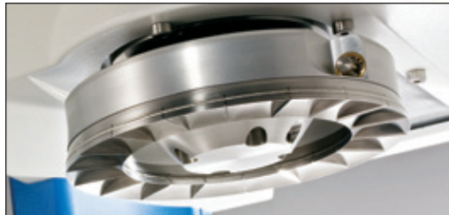
Close-up View of Vane Lid used for Flow Function Test.
